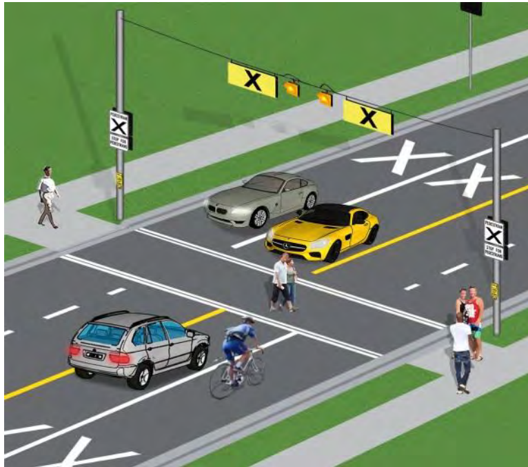
Figure 1 Level 1, Type 1 Pedestrian Crossover
